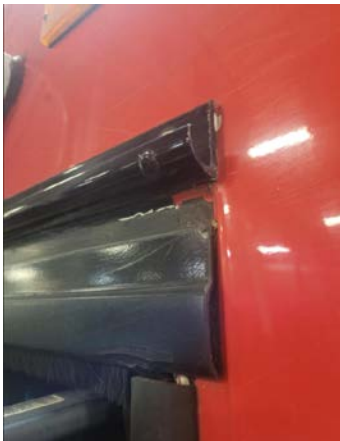
Figure 8. Drip Rails and Window frames
