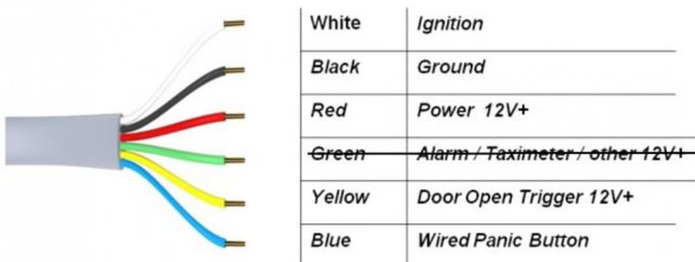
IDrive Wiring Diagram
