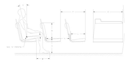
Seat dimensions for the various seating arrangements shall have the dimensions as follows (refer to Figure 10):
