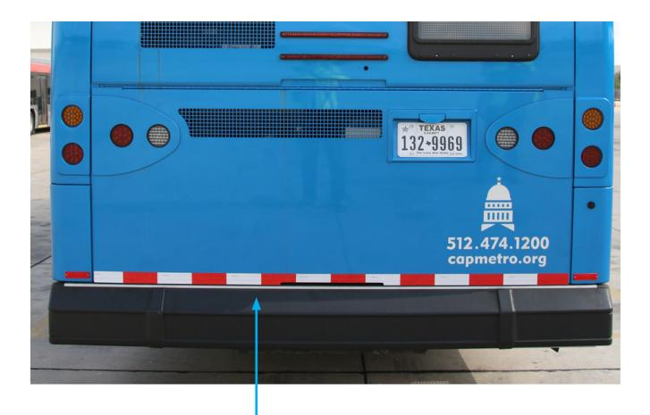
Apply tape below the tail lights, across the bottom of engine compartment
