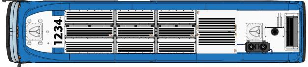
Roof Number/ Vinyl Decal: 15"height, centered on roof font: Geometric 415 Black 3M Scotchlite Reflective Black 680-85
