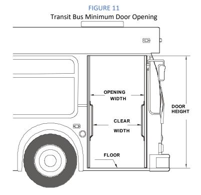
When open, the doors shall leave an opening no less than 75 inches in height. Front door clear width shall be a minimum of 32 inches with the doors fully opened. Rear door opening clear width shall be a minimum of 40 inches with the doors fully opened.
